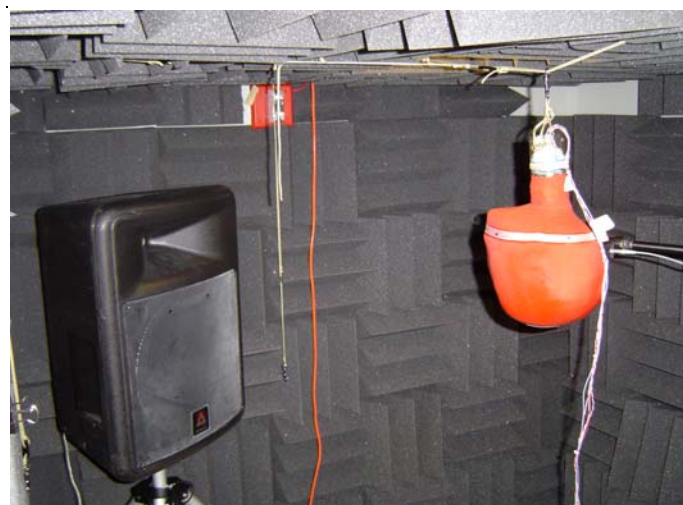
Figure 4. Head Simulator Mounted in the Acoustic Test Facility. Simulator is inverted and suspended approximately 1 m from the sound source.
