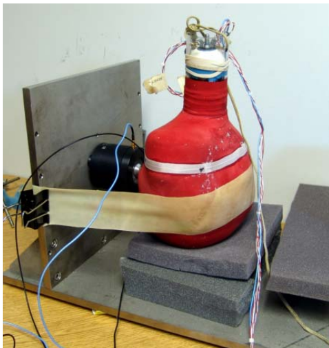
Figure 3. Driving Point Impedance Test Setup. The head simulator is held against a shaker using latex bands.
